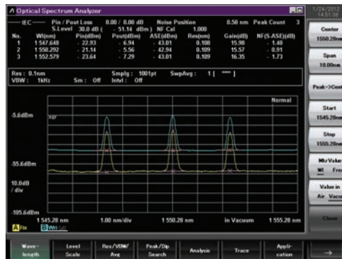
Example of Opt. Amp (Multi-channel) Analysis Function Measurement
